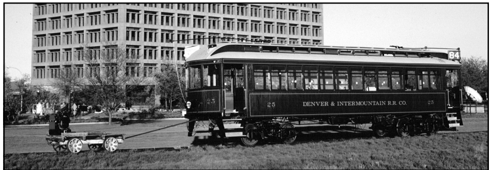
On May 2nd, No. 25 ventures away from Building 78 for the first time since its arrival at the Denver Federal Center in December of 1988. Tom Gill's portable welder provides the initial power supply for this test run as it passes by the Bureau of Reclamation Building.
